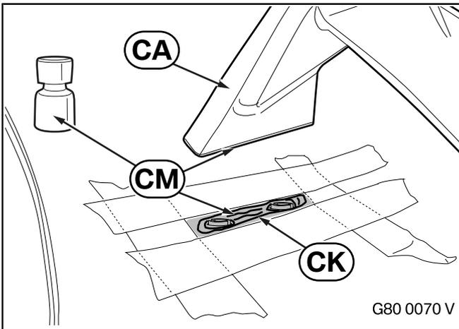
Apply the primer **CM** to both surfaces. Wait until the drying time has elapsed.
