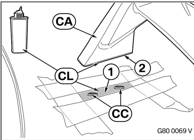
Abrade the surface (1) the boot lid and the surface (2) the boot lid spoiler **CA** using suitable equipment, but do not abrade the heads of the adjustment sleeves **CC**.
