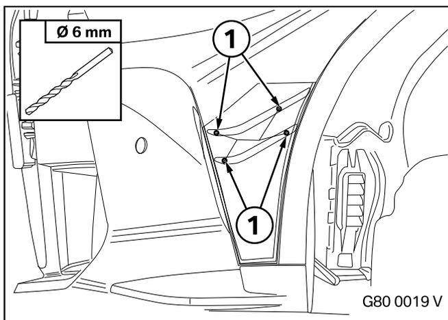
☐ Be careful not to damage the components underneath when drilling holes. ◀
