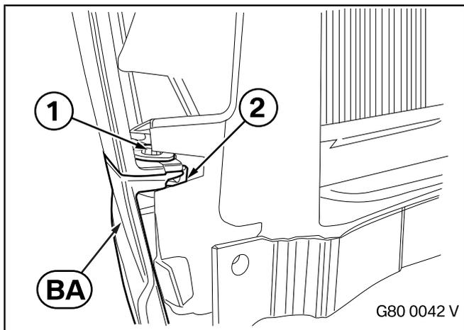
▶ After around 24 hours, as soon as the liquid adhesive is dry, remove the adhesive tape and spacer and carry out the following step.
