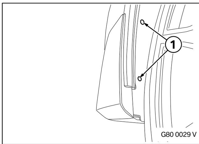
Tighten the existing screws (1) in the wheel arch trim.
