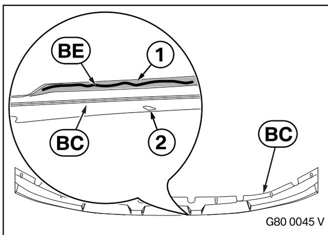
Abrade the internal surface (1) against the holes (2) in the centre front attachment **BC** over the full width of the component on the external edge using suitable tools and clean it with cleaner **BF**.
