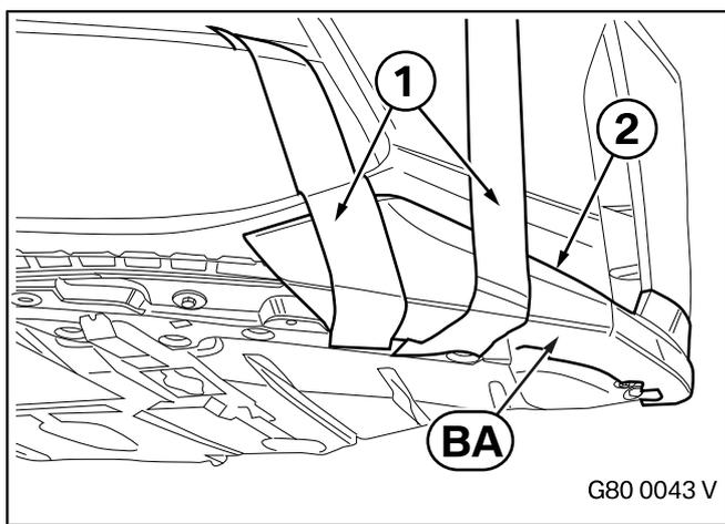
Remove any excess liquid adhesive immediately using suitable equipment. ◀
