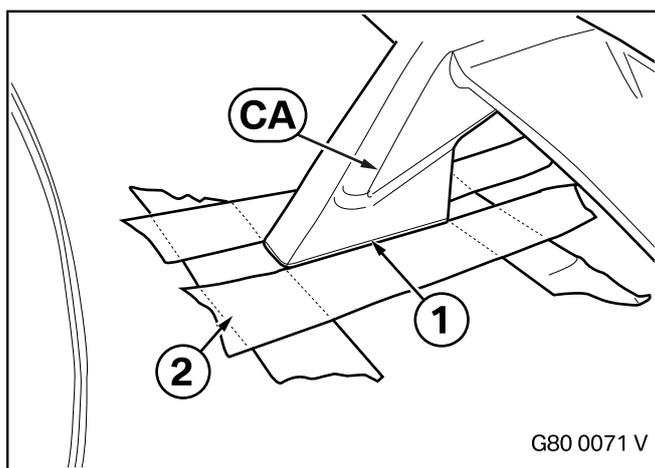
Remove excess liquid adhesive immediately using suitable equipment and dab the joint (1) with suitable equipment (for example cotton buds).
