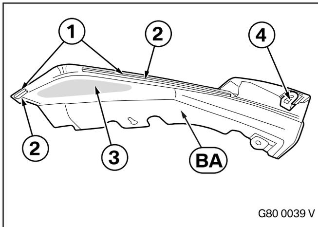
Abrade the narrow surface (1) above the adhesive tapes (2) on the inside of the right front attachment **BA** using suitable tools.
