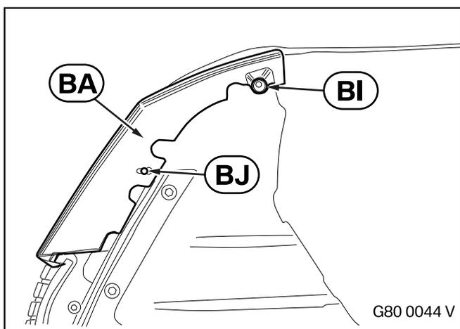
Press the expanding rivet **BI** into the right front attachment **BA**.
