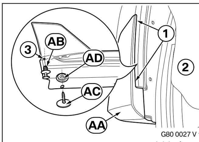
▶ As you tighten the hexagon screw **AC** and the plastic cap nut with washer **AD**, ensure that there is a uniform gap (1) between the winglet and the car. ◀
