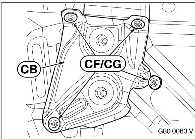
Secure the holder plates **CB** to the boot lid using four M5x16 screws **CG** and four washers **CF** on each side of the car.
