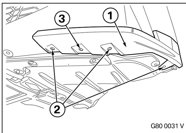
Remove the two side trims (1) as described in **ISTA/AIR**. Keep the expanding rivet (2) and screw (3); they will be reused later.
