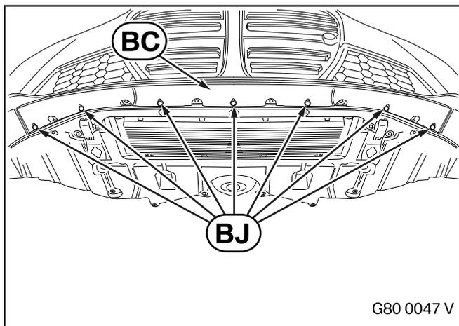
Insert the expanding rivets **BJ** into the oval holes in the centre front attachment **BC** as far as possible to the rear of the oval holes and press them firmly into place.
