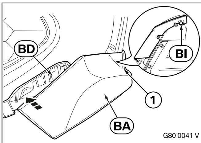
Position the right front attachment **BA** on the outside around the wheel arch (1) on the front apron and insert the expanding rivet **BI** at the rear without initially creating any adhesive contact. Now turn the right front attachment **BA** to the front on the apron and glue it to the underbody console **BD** and front apron.
