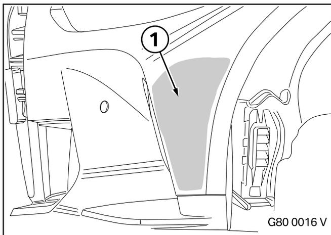
☐ The bonding surface must be completely dry, clean, and free from wax or grease. ◀
