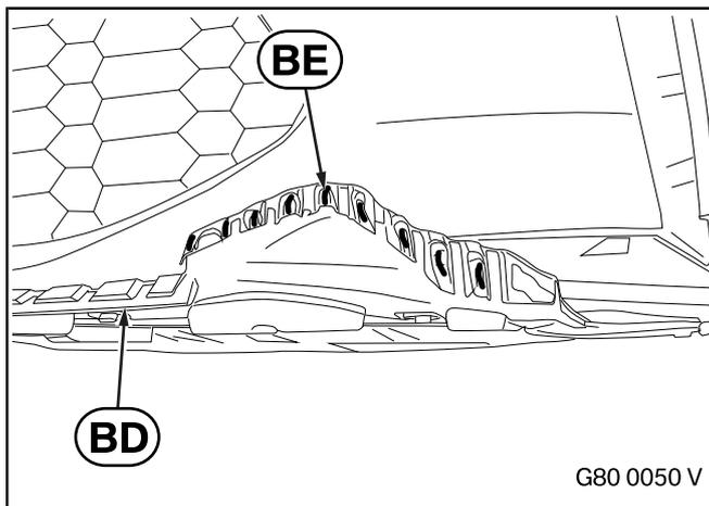
Apply the liquid adhesive **BE** to the surface of the underbody console **BD**.
