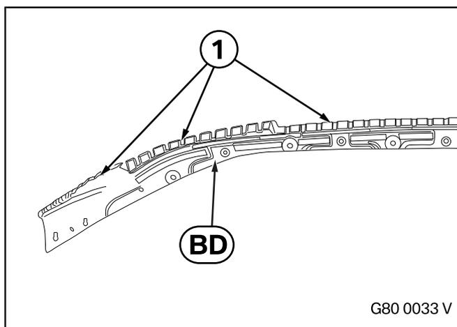
Abrade the surfaces (1) on the top of the underbody console **BD** using suitable tools and clean them with cleaner **BF**.
