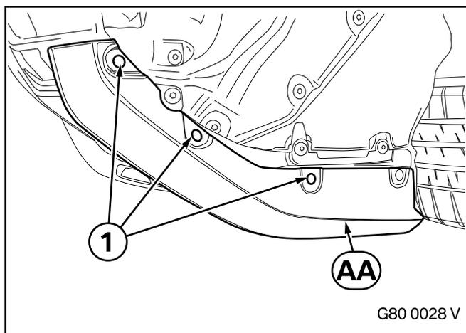
Now press the three existing expanding rivets (1) fully into the rear winglet **AA**.
