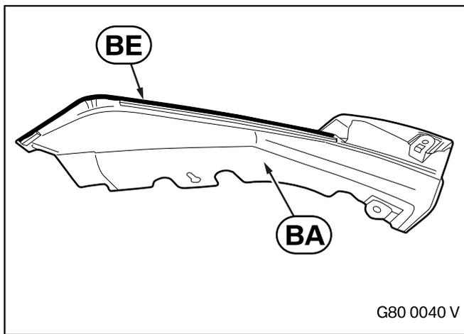
Apply a bead of the liquid adhesive **BE**, see black line in the figure at the top edge.
