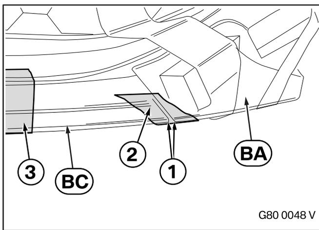
Position the centre front attachment **BC** in the middle between the two front attachments **BA** and **BB** so that there is a uniform gap on the left and right (1) and the surfaces fit together to create a smooth finish. Secure the spacer and the gap using suitable adhesive tape (2).
