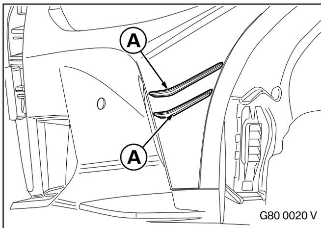
Position the flicks **A** and check their contours. Re-work the holes if necessary.
