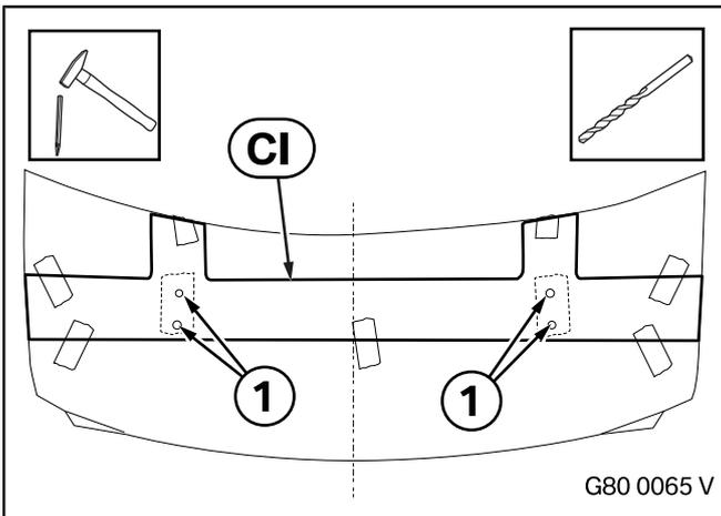
Centrepunch the four marked holes (1) on the drilling template **CI**.
