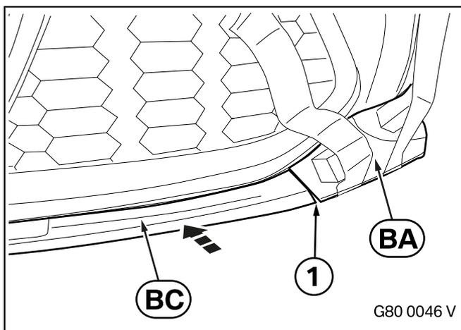
Install the centre front attachment **BC** in the middle between the two side parts. To do this, push the component from above onto the underbody console to prevent the liquid adhesive smearing (slide it downwards along the front apron).
