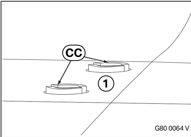
Adjust the adjustment sleeves **CC** from outside. Unscrew them until the heads are above the external skin of the boot lid and the external skin of the boot lid (1) is moved upwards slightly by the sealing rings **CD**.
